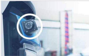
Small and unobtrusive cameras were fitted to key spots on Martin Ryan's trucks, giving them a 360° view of the vehicle.
